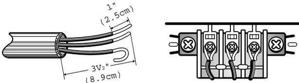
1. Loosen or remove center terminal block screw.
