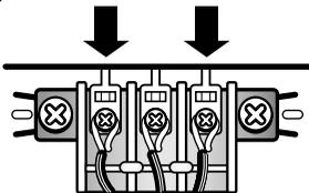
4. Tighten strain relief screws.
