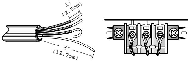
1. Remove center terminal block screw.
