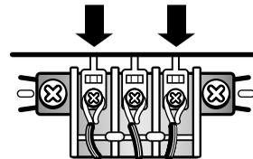
4. Tighten strain relief screws.
