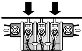
6. Tighten strain relief screws.
