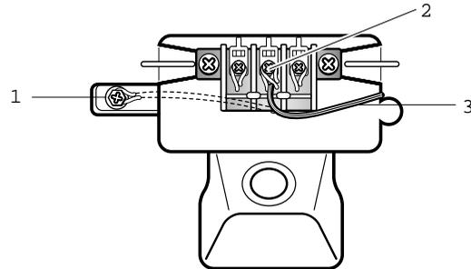
1. External ground connector - Dotted line shows position of NEUTRAL ground wire before being moved to center terminal block screw
