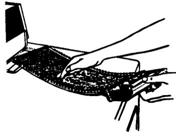
3. Do not rinse or wash the lint screen to remove lint. Wet lint can clog the screen mesh.
