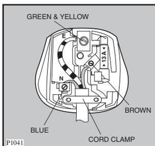
The wire coloured green and yellow must be connected to the terminal marked with the letter «E» or by the earth symbol  $\equiv$  or coloured green and yellow.
