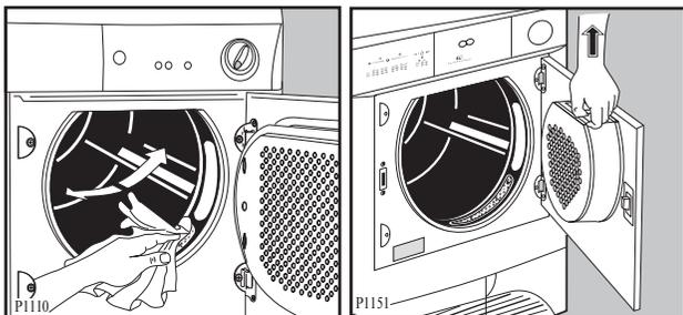
The filter in the inner door must be removed for cleaning. Do not be alarmed by the amount of fluff. It is not due to excessive wear caused by the dryer. All fabric loses fluff when drying but it goes un-noticed in the air. In a tumble dryer it simply collects in the filter.
