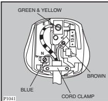
If you fit your own plug, the colours of the wires in the mains lead of your appliance may not correspond with the markings identifying the terminals in your plug.
