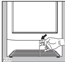
To pull out the condenser, first turn the two red stops downwards as shown below and then remove the condenser unit holding it with the handle.
