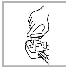
! The plug must not be used without the fuse cover in place. If a replacement fuse holder/cover is required, it must be of the same colour coding or wording as shown on the base of the plug. Replacements are available from authorised dealers.
