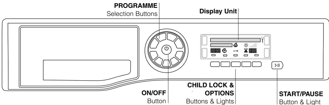
The **ON/OFF** button - if pressed when the dryer is running: If the display shows **TURNING OFF** the dryer stops. If the display shows **PRESS AND HOLD** hold the button and the display counts down 3, 2, 1 and then stops.
