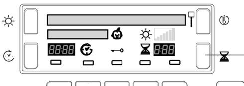
After selecting a programme that has a Timed Dry option, press the ⏰ Timed button and the display will increment the selected time, each time you press and release the button (see *Start and Programmes*).
