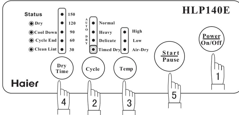
**1 Press in the 'PowerOn/Off' button to run the machine.**
