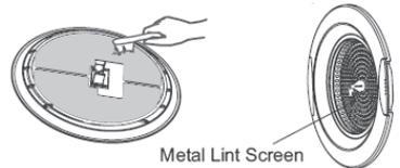
**3. Re-installing the filter**
