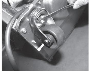
**Note:** Two of the casters include locking mechanisms to ensure the unit does not slide on hard floors. These two locking casters should be fastened at the front end of the unit, with the unlocked casters fastened on the rear end.
