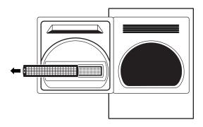
**The Exhaust Duct:** Inspect and clean the exhaust ducting at least once a year to prevent clogging. A partially clogged exhaust can lengthen the drying time.
