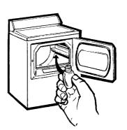
Before replacing the light bulb, be sure to unplug the dryer power cord or disconnect the dryer at the household distribution panel by removing the fuse or switching off at the circuit breaker. Reach above dryer opening from inside the drum. Remove the bulb and replace with the same size bulb.
