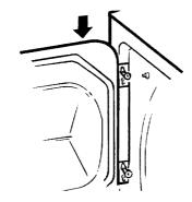
7 Remove the remaining screws from the side of the opening from which the door was removed. With these screws secure each hinge at the bottom.
