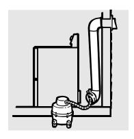
Inspect and clean the dryer exhaust ducting at least once a year to prevent clogging. A partially clogged exhaust can lengthen the drying time.
