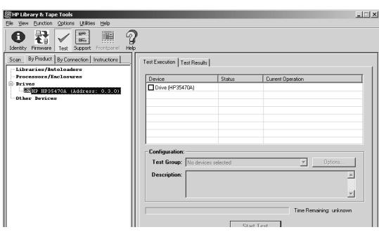
If you are upgrading to a new drive technology, use HP StorageWorks Library and Tape Tools to upgrade the library firmware before installing the new tape drive.
