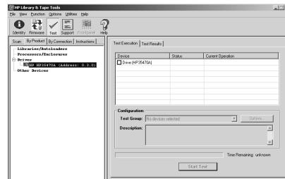
Use HP StorageWorks Library and Tape Tools, Remote Management Interface (RMI), or MSLUtil diagnostic software to upgrade the drive to the latest firmware.
