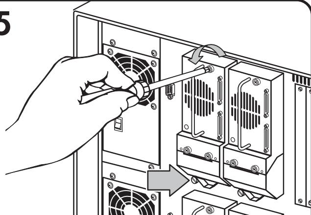
Using a flat-blade screwdriver, loosen the two captive thumbscrews at the top center and lower left of the tape drive.
