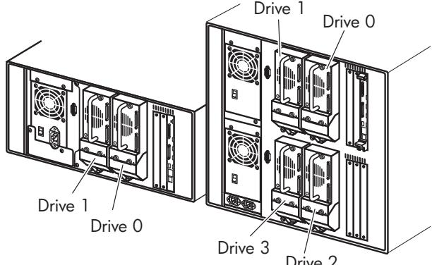
Unload any tape cartridges in the drive to be removed using your application software or the library GUI touch screen.
