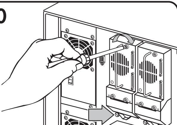
Using a flat-blade screwdriver, tighten the two captive thumbscrews. If adding an additional drive, configure the library for the new tape drive. Refer to the tape library user guide for more information.
