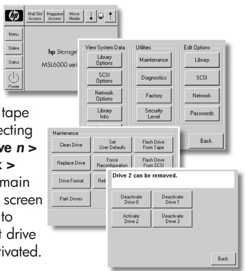
Activate the tape drive by selecting **Activate Drive n > Back > Back > Back** to the main screen. The screen will change to indicate that drive n is now activated.
