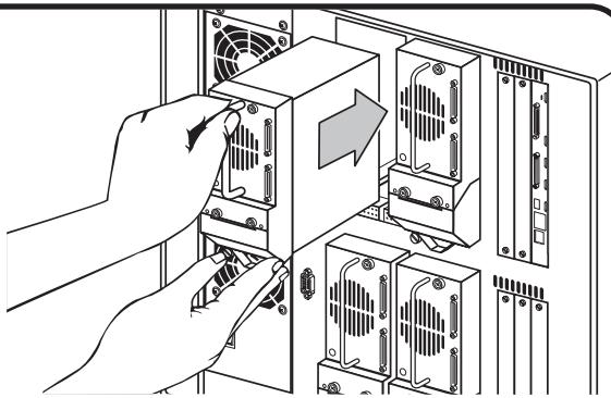
Slowly insert the new tape drive into the drive bay, aligning the connectors on the tape drive with the connectors in the drive bay.
