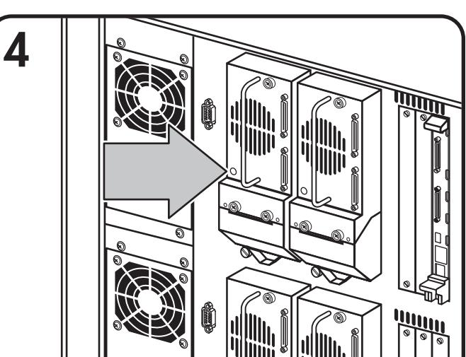
Make sure that the LED on the tape drive to be removed is off.
