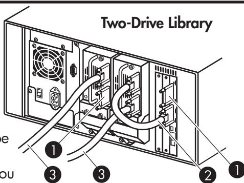
If you are adding an additional tape drive to your library, or if you are upgrading an existing drive, ensure you use supported cabling configurations. See the *HP StorageWorks MSL6000 Series Tape Library User Guide* for more information. The user guide can be downloaded from <http://www.hp.com/support>.
