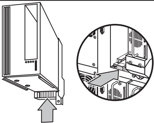
Before installing the new drive, inspect the connectors on the tape drive and in the drive bay. Ensure that the connectors are intact, free of any foreign objects, and have no cracks or deformed contacts.
