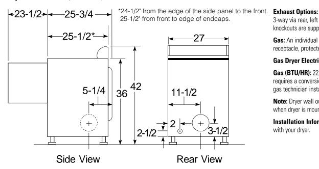
3-way via rear, left and bottom. Dryer is shipped exhausted to the rear. Alternate exhausting knockouts are supplied.
