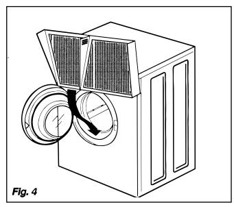
Never operate the dryer without the lint filter in place.
