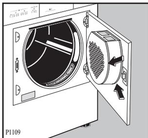
If necessary the filters can be cleaned under running water using a brush. In this case, remove the filter in the door opening as per picture (it can be positioned with the tongue facing to the left or to the right).
