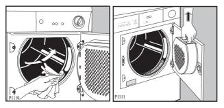
The filter in the inner door must be removed for cleaning. Do not be alarmed by the amount of fluff. It is not due to excessive wear caused by the dryer. All fabric looses fluff when drying but it goes un-noticed in the air. In a tumble dryer it simply collects in the filter.
