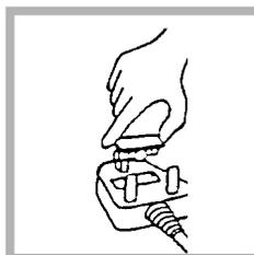
! The plug must not be used without the fuse cover in place.
