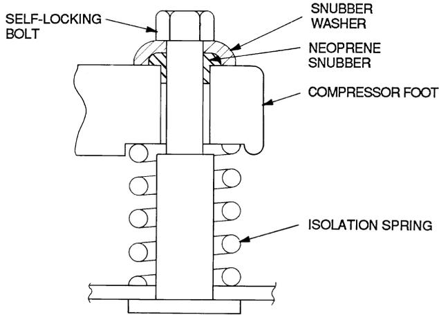
**Fig. 4 — Typical Compressor Mounting (38AKS Units)**
