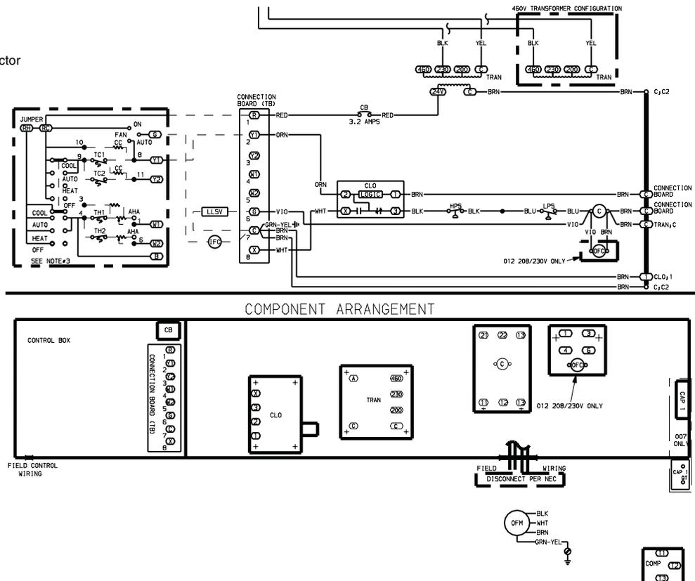
**Fig. 6 — Typical Control Wiring Connections/Component Arrangement (38AK Shown)**
