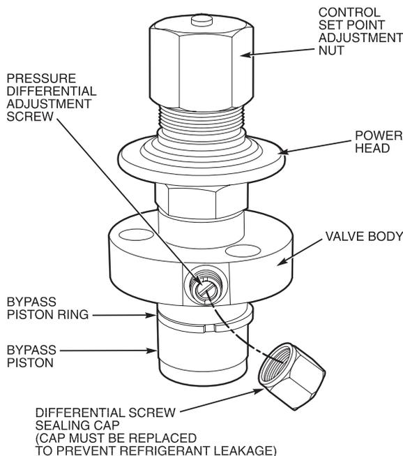
**Fig. 14 — Compressor Capacity Control Unloader**
