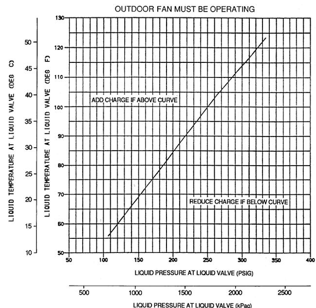
**Fig. 8B — Cooling Charging Chart — 38AK007 (50 Hz)**
