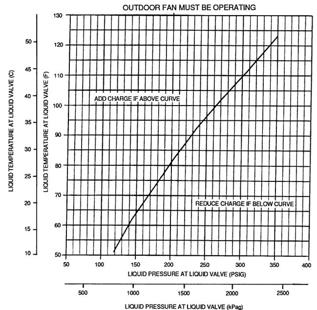
**Fig. 8A — Cooling Charging Chart — 38AK007 (60 Hz)**
