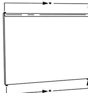
13. Remove the screw in the top right corner of the bottom panel. (If you have a condenser dryer, you will have to open the condenser unit door.)
