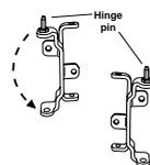
6. Transfer the top hinge pin to the right side of the dryer casing.
