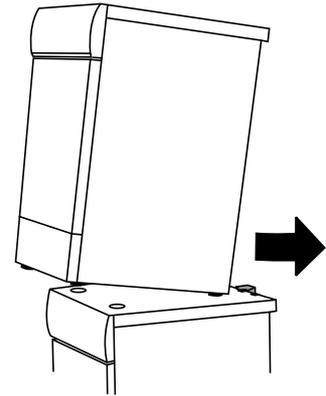
6. Carefully lower the front of the dryer, making sure the feet fit into the plastic cups.
