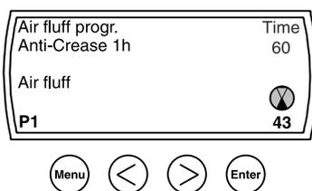
The remaining time toggles between the minutes remaining (e.g., 23) and the hour(s) remaining (e.g., 1h).
