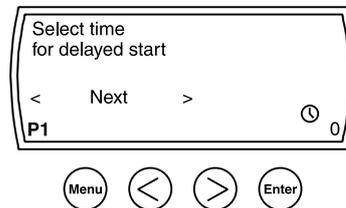
2. In the bottom right corner of the LCD window, a clockface and a zero will flash. To change the zero, simply press an **Arrow** button until the LCD displays the number of hours you want to delay starting the program (1–24 hours).
