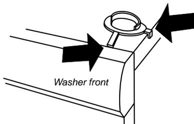
4. Once the cups are correctly in place, break off the remaining plastic tabs.
