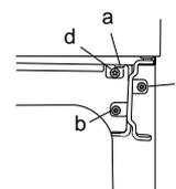
16. Replace the screw you removed in step 13 (d).
