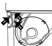
3. Supporting the door from the bottom, pull it out and to the left as you turn the hinge bracket counter-clockwise.
