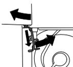
4. Remove the hinge pin at the top of the hing bracket.
