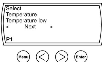
2. Use the **Arrow** buttons to toggle between the Normal and Low temperature settings.
