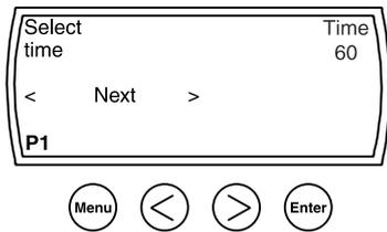
2. To change the number, simply press an **Arrow** button until the length of time you want the program to run displays.
