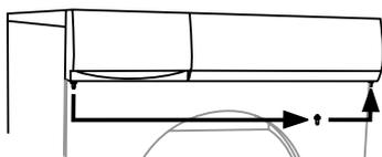
7. Loosen the two screws on both outer edges of the door so you can remove the magnetic door catch and the cover plate.
