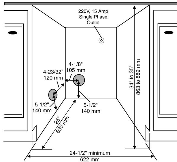
**NOTES:** The height adjustment for the dryer is 33-1/2" to 34-1/2" (850 mm to 876 mm). Do not raise it higher than 34-1/2".
