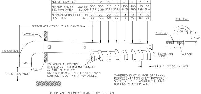
IMPORTANT: NO MORE THAN 8 DRYERS CAN BE CONNECTED TO ONE COMMON DUCT ( VENT ).
