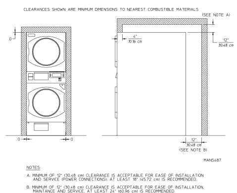
**IMPORTANT:** Dryer *should be* located where a minimum amount of exhaust duct <u>will be</u> necessary.
