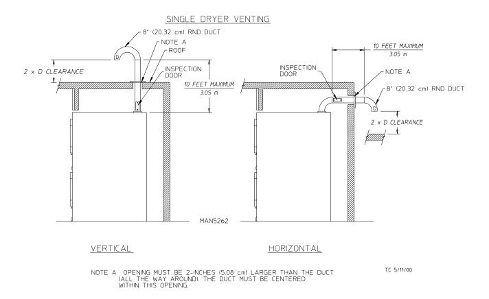
**IMPORTANT: DO NOT** use screens or caps on the outside opening of the exhaust duct work.
