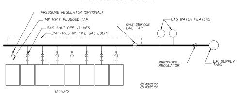
**WARNING:** Test <u>ALL</u> connections for leaks by brushing on a soapy water solution (liquid detergent works well).
