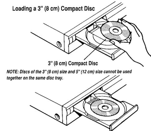
NOTE: Discs of the 3" (8 cm) size and 5" (12 cm) size cannot be used together on the same disc tray.
