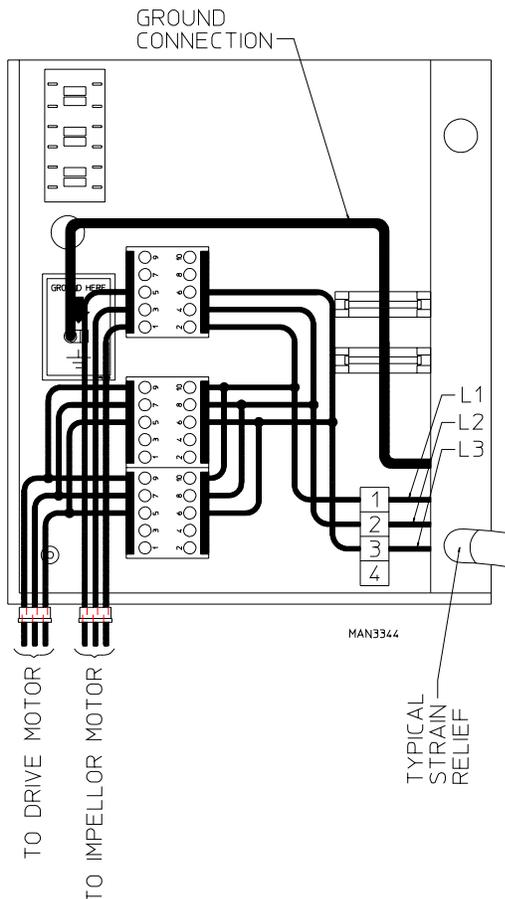
For gas dryers and steam dryers manufactured for operation at 3-phase (3 $\phi$ ), the electrical connections are made at the power distribution block located in the service box at the rear, upper left corner of the dryer. The ground connection is made to the copper lug also provided in this box. To gain access to the service box contactor, the service box cover **must be** removed.
