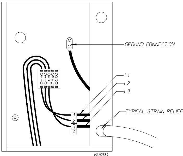
If local codes permit, power to a gas dryer or steam dryer can be made by the use of a flexible U.L. listed power cord or pigtail (wire size **must conform** to rating of dryer), or the dryer can be hard wired directly to the service breaker panel. In **ALL** cases, a strain relief **must be** installed where the wiring enters the dryer and service box area.
