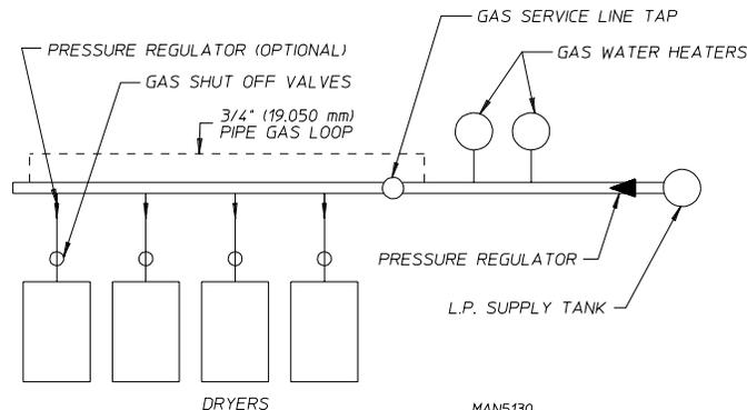
Consistent gas pressure is essential at **ALL** gas connections. It is recommended that a 3/4-inch (19.05 mm) pipe gas loop be installed in the supply line servicing a bank of dryers. An in-line pressure regulator **must be** installed in the gas supply line (header) if the (natural) gas pressure exceeds 12.0 inches (29.9 mb) of water column (W.C.) pressure.
