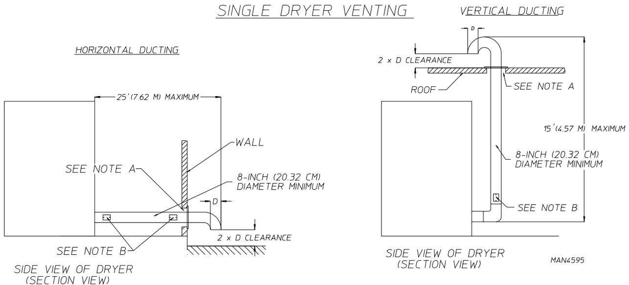
NOTE: "A"- OPENING MUST BE TWO (2) INCHES (5.08 CM) LARGER THAN DUCT (ALL THE WAY AROUND). THE DUCT MUST BE CENTERED WITHIN THIS OPENING.
