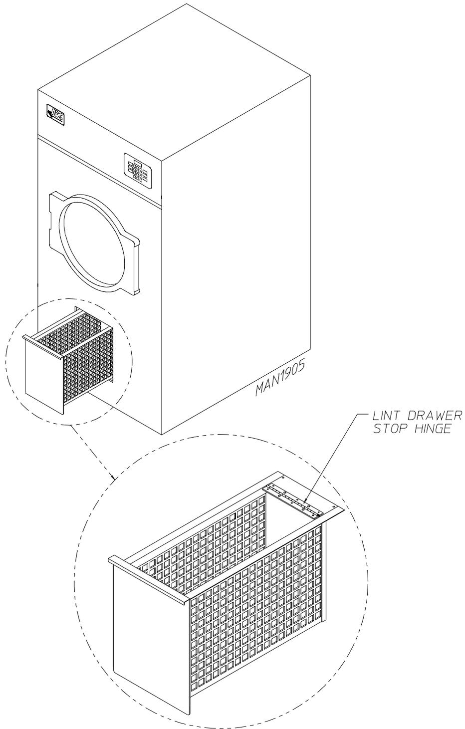
**IMPORTANT:** After replacing the lint drawer back into the dryer, be sure to rotate/move hinge back to the upward stop position.
