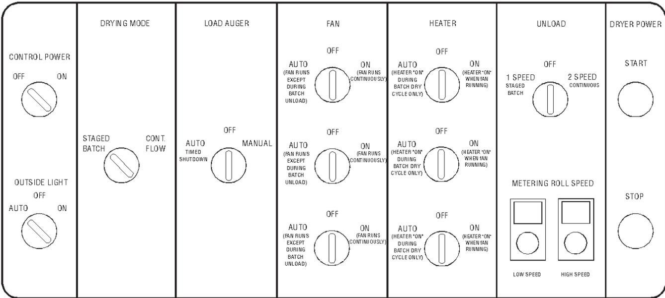
Figure 1: The grain dryer control panel with the Electronic Monitoring Control System in the upper right panel.
