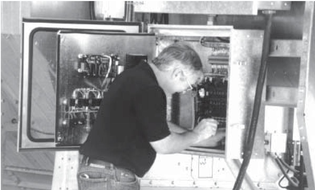
Airstream Service Technician checks the wiring on a single module grain dryer.
