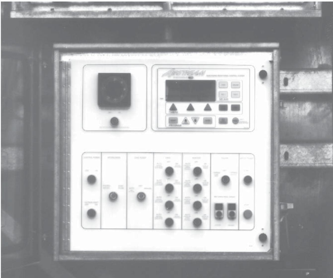
The Airstream Dryer Control Panel mounted on the dryer.
