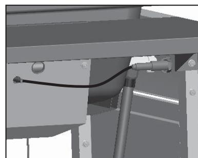
**13** Attach lower lid hinges to back of firebox using two **#10-24X1/2"** machine screws, **fiber washers** and **#10-24 flange nuts** per hinge. Center flat portion of hinge should be on bottom (see inset below).
