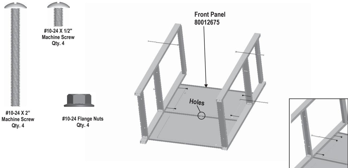
**3** Turn cart assembly over and attach lower rear panel to legs using four #10-24 X1/2" machine screws.
