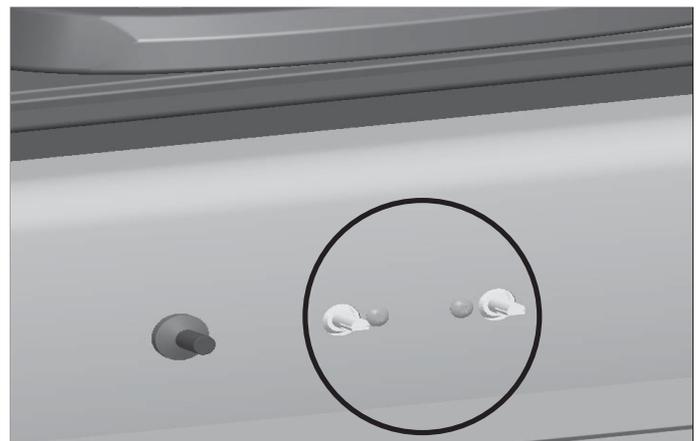
5. If “growing” bubbles appear, there is a leak. Close LP cylinder valve immediately and retighten connections. **If leaks cannot be stopped do not try to repair.** Call for replacement parts. Order new parts by giving the serial, model number and name and part number of items needed (see parts list) to the Grill Service Center at 1-800-241-7548.
