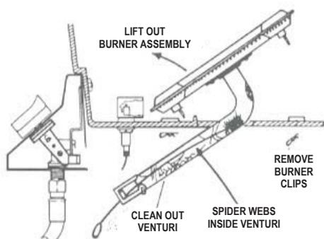
In some areas of the country, spiders or small insects have been known to create "flashback" problems. The spiders spin webs, build nests and lay eggs in the grill's venturi tube(s) obstructing the flow of gas to the burner. The backed-up gas can ignite in the venturi behind the control panel. This is known as a flashback and it can damage your grill and even cause injury.
