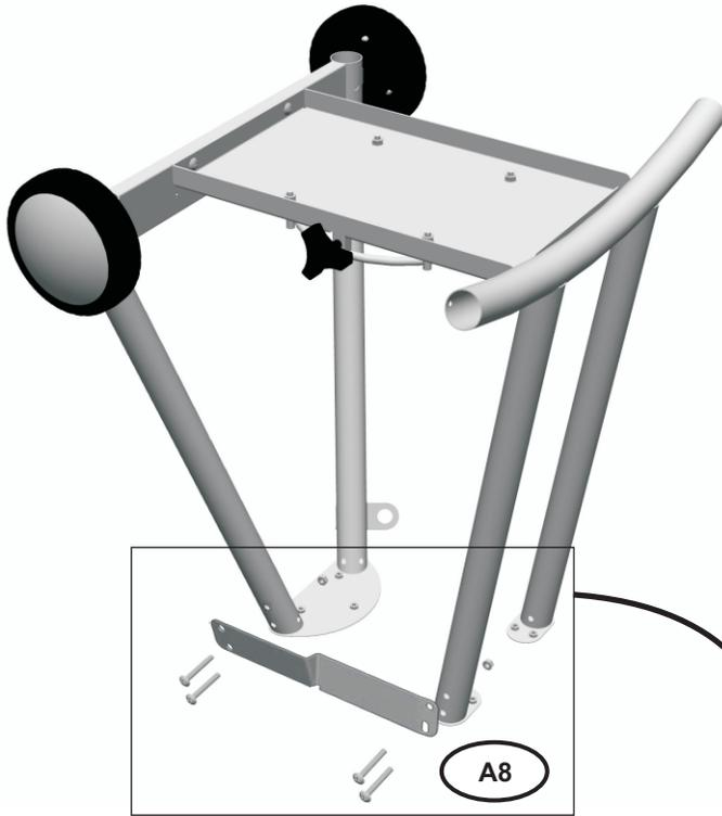
**Step 3** - Carefully turn the **Cart Assembly** over and allow it to rest on the tops of the leg assemblies. Assemble the **Cart Bracket (A8)** to the **Cart Assembly** by inserting 4 each **1/4-20x2"** screws into corresponding holes as shown. Allow the **Cart Bracket** to rest on the floor, this will help with alignment. Secure with 4 each, **1/4-20 nuts** using a small adjustable wrench, not supplied. **FINGER TIGHTEN ONLY AT THIS TIME.** The bracket will be tightened in step B2.
