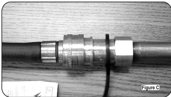
With proper assembly, the gas hose cannot be removed without pushing the quick disconnect sleeve back. To disconnect, push sleeve back and pull plug out of sleeve (this automatically shuts off gas).
