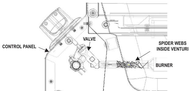
In some areas of the country, spiders or small insects have been known to create "flashback" problems. The spiders spin webs, build nests and lay eggs in the grill's venturi tube(s) obstructing the flow of gas to the burner. The backed-up gas can ignite in the venturi behind the control panel. This is known as a flashback and it can damage your grill and even cause injury.
