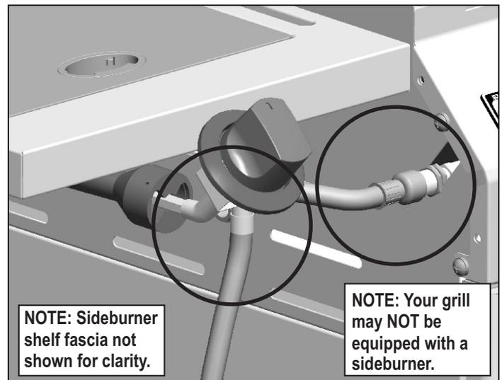
5. If “growing” bubbles appear, there is a leak. Close LP cylinder valve immediately and retighten connections. **If leaks cannot be stopped do not try to repair.** Call for replacement parts.
