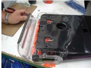
Turn the machine on its side so that the belt access area is facing upwards. Making sure the cord side of the machine is facing down
