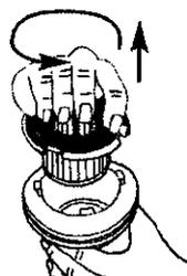
Remove filter from filter/float assembly by grasping angled top of filter and turning counterclockwise. Lift filter up and out of filter assembly.
