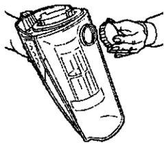
Remove measure cap from the rear of the Clean Water Tank. Pour 4 capfuls of Kenmore® Hard Floor Concentrate Cleaner into Clean Water Tank. **DO NOT USE PINE, SOLVENT, OR WAX BASED CLEANING SOLUTIONS IN CLEANER.**
