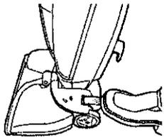
Step on Nozzle Setting pedal if necessary to switch from HARD FLOOR DRY VAC to WET SCRUB & VAC position.
