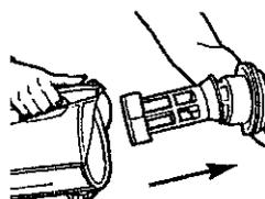
Grasp tab on filter/float assembly and pull up to remove from tank.
