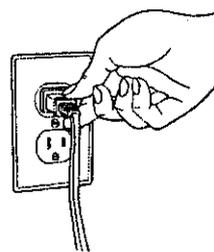
With dry hands, plug cord into properly grounded electrical outlet.
