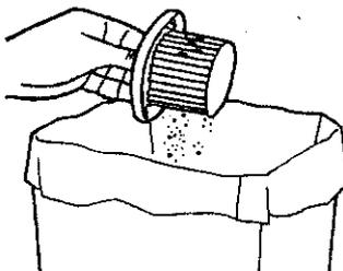
Remove any loose debris from filter by tapping the filter against a garbage can. **NOTE:** For additional cleaning, the filter may be rinsed under water (Diagrams a and b). Allow filter to air dry completely before use.
