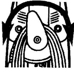
1. Turn the quick release upper cord hook to either side and down to release the power cord.
