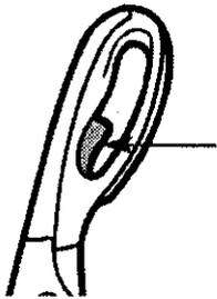
Pull Solution Trigger to start the flow of cleaning solution.
