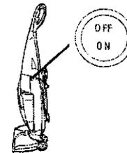
Turn cleaner on by moving power on/off switch from OFF to ON.
