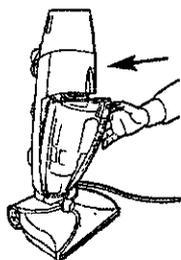
Replace Tank-in-Tank™ System by inserting bottom first and tilting forward until tank latch fastens.
