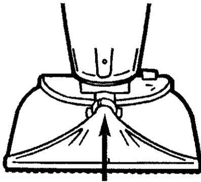
Insert new nozzle by pushing securely into Nozzle Lock. **NOTE:** Make sure nozzle is inserted all the way in the Nozzle Lock, otherwise Nozzle Lock will not secure properly. Failure to install nozzle correctly can impact cleaning performance.
