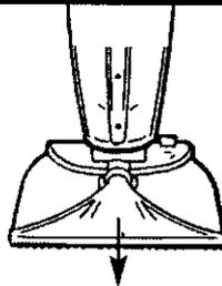
Pull nozzle forward to remove completely from Nozzle Lock.
