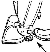
Step on Nozzle Setting pedal if necessary to switch from WET SCRUB & VAC to HARD FLOOR DRY VAC.
