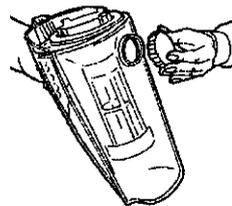
Remove measure cap from the rear of the Clean Water Tank. Pour 2 capfuls of Kenmore® Carpet & Upholstery Concentrate Cleaner into Clean Water Tank.
