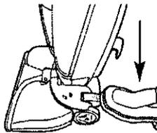
Step on Nozzle Setting pedal if necessary to switch from HARD FLOOR DRY VAC to WET SCRUB & VAC.
