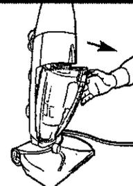
Remove Tank-in-Tank™ System by pushing down on tank latch and tilting out from cleaner.
