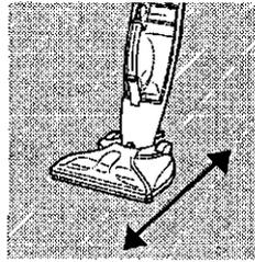
With solution On/Off trigger held down, slowly push unit forward. Release solution On/Off trigger and pull unit backward in the same area cleaned to remove dirty water and solution from hard floor. Overlap strokes by one inch to prevent streaking. (For heavily soiled areas, repeat if necessary).
