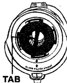
Grasp tab on filter/float assembly and pull up to remove from tank. Empty contents of Dirty Water Tank.
