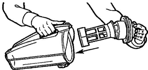
Return filter/float assembly to Dirty Water Tank. To ensure proper fit, make sure the arrow on the filter/float assembly lines up with the Align Filter Front arrow on Tank-in-Tank™.
