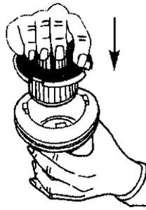
Replace filter by grasping angled top of filter and turning clockwise to lock onto filter/float assembly.
