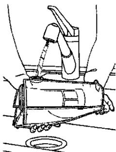
Fill remainder of Clean Water Tank with warm water up to the MAX FILL line. Replace measure cap on Clean Water Tank.
