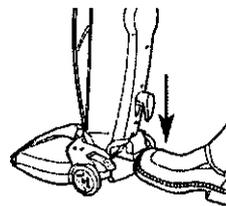
Step on Handle Release pedal to put into cleaning position.
