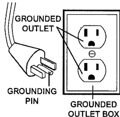
This appliance is for use on a nominal 120-volt circuit and has a grounding attachment plug that looks like the plug illustrated in the sketch above. Make sure that the appliance is connected to an outlet having the same configuration as the plug. **No adapter should be used with this appliance.**
