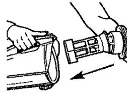
Return filter/float assembly to Dirty Water Tank. To ensure proper fit, make sure the arrow on the filter/float assembly lines up with the Align Filter Front arrow on Tank-in-Tank™.
