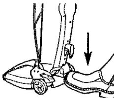
Step on Handle Release pedal to put into cleaning position.
