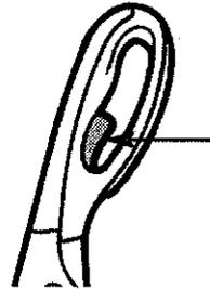
Pull Solution Trigger to start the flow of cleaning solution. **NOTE:** Cleaner will continuously dispense solution until Solution Trigger is released.
