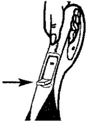
Slide Brush On/Off switch to the ON position.
