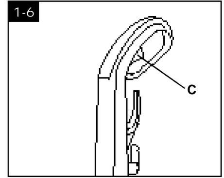
**When handle sections are completely together, squeeze trigger (C) on upper handle.**
