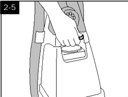
The deep cleaner may also be lifted by placing a hand under the upper clean solution tank handle as shown.
