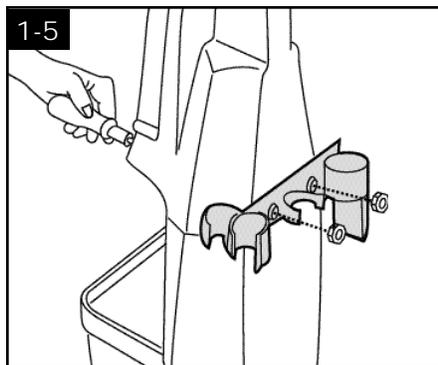
Place **nuts** in recessed areas on **back of the hose holder**. Hold each nut in place while tightening each bolt securely (from the front of the handle) with a Phillips screw driver.
