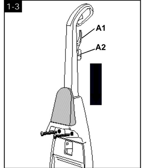
With hose hook (A1) and cord hook (A2) to back of deep cleaner, push upper handle down onto lower handle. Push **bolts** into holes on **front of handle**. If bolts will not go through hole easily handle is not pushed completely down.
