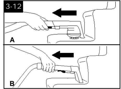
9. Lift tool, and position it against riser. Pull tool **slowly** over carpet without pressing trigger (dry stroke). It is best to alternate wet and dry strokes as described above. End with more dry strokes to aid in faster drying of carpet.
