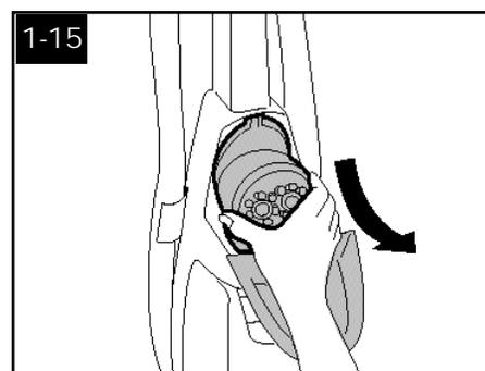
To remove powered hand tool, pull it down and outward.
