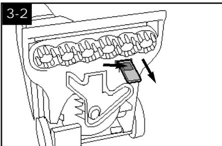
**e.** Remove lint from filter screen located on bottom of cleaner as follows. **Note: When brushes seem to be rotating slowly, disconnect deep cleaner from electrical outlet and check and clean this screen.**
