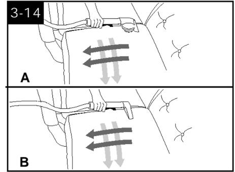
10. For heavily soiled areas, it may be necessary to repeat the cleaning process. Make crisscrossing strokes to the original pattern; overlap each pass.
