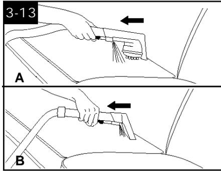
6. Gently press the tool onto the fabric. Press the trigger and slowly pull the nozzle over the fabric.
