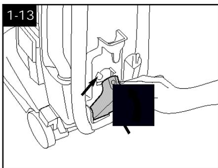
Position stair/upholstery nozzle in holder at base of cleaner and snap it into place as shown at arrow.
