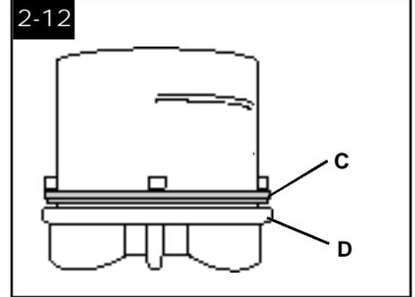
If rubber ring (C) on cap has become dislodged, reposition it with uneven side against ledge (D) as shown.
