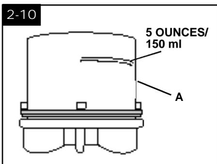
Turn cap (A) upside down to serve as a measuring cup. Using cap, measure detergent following the chart below.
