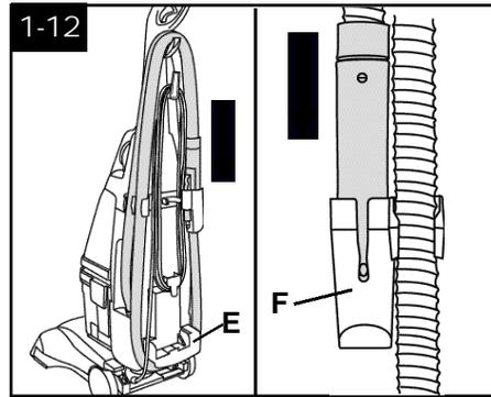
Continue wrapping hose under lower hook (E). Snap hose end **fully** into holder (F).
