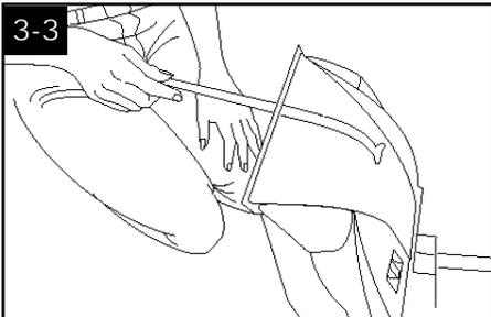
A nozzle clean-out tool, available at additional cost if not included with your cleaner, can be used for removing debris or if a non-carpeted floor is not available.
