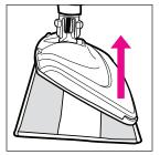
When unit has cooled, remove Ultra-microfiber pad. Store unit upright in a dry area.
