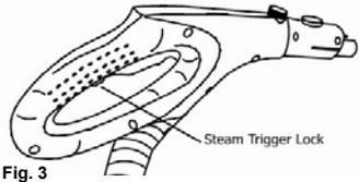
**WARNING:** This appliance is under pressure. After every use, unplug the unit and press the steam trigger button until all pressure has been released before removing safety cap. Allow unit to cool for fifteen (15) minutes before refilling.
