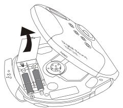
**Note**: To prevent loss the battery cover cannot be completely removed from the player.
