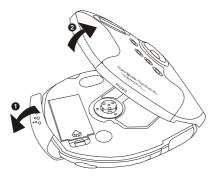
Remove the "dummy CD" transit protection card from the CD spindle and discard it.
