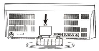
2.) Install 3 fresh "AA" alkaline batteries in the battery compartment. Be sure to install the batteries correctly, according to the polarity (+ / -) markings inside the battery compartment.
