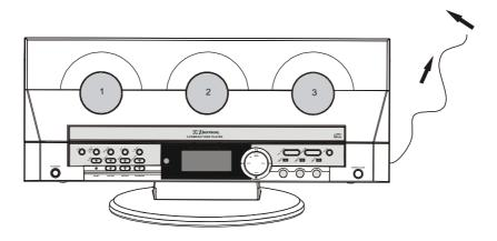
AM: The AM bar antenna is inside the cabinet of the main unit. You may need to change the position of the main unit until you find the position that provides the best reception for your favorite AM stations.
