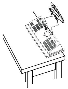
3.) Return the main unit and the pedestal base to the upright position and slide the main unit all the way backward in the direction of the 'arrow' onto the pedestal until the locking tabs 'click' and the main unit is locked in place.
