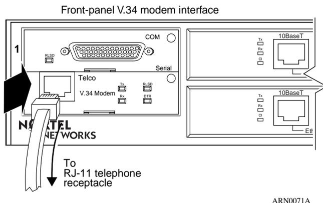
**Figure 1-1. ARN V.34 Modem Adapter Module Connector (Slot 2)**
