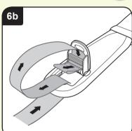
the harness strap down over the bar of the SAFESTRAP<sup>™</sup> mechanism and pull through (dia 6b).
