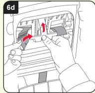
Push the chest pad strap through the shoulder strap slot towards the back of the seat. Attach the chest pad strap to the chest
