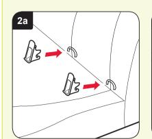
Installing the child seat If required, clip the two insertion guides onto the two ISOFIX anchorage points on the vehicle seat (between seat and backrest). The cut out on the insertion guide must point upwards (dia 2a). The insertion guides should be removed when not in use.
