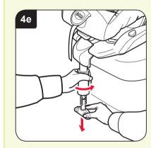
Turn the foot prop handle anticlockwise **①** and pull out the foot prop **②** until it rests firmly on the floor of the vehicle (dia 4e). **IMPORTANT** – The foot prop must never be suspended in mid-air or supported by other objects. Also ensure that the foot prop does not raise the child seat from the vehicle seat surface.
