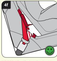
**IMPORTANT** – After installing the child seat you need to check the position of the seat belt buckle. Checking the position of the seat
