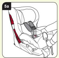
Push the adjuster button in and at the same Turn the seat around and open the User time pull **BOTH** shoulder straps forward as Guide storage flap. Lift the harness adjuster far as possible (dia 5a).
