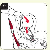
To adjust the height of the headrest and harness to fit your child: Loosen the harness straps as far as
