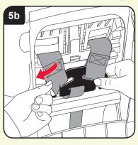
at the back of the seat shell and move it up so that the shoulder strap slots in the headrest are in the top position. Unhook the harness strap from the yoke at the back of the child seat. Pull the harness strap through the shoulder strap slot to the front of the seat (dia 5b).
