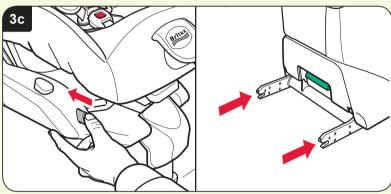
Press and hold the tension button whilst pushing the catch arms into the seat base at the same time (dia 3c). Fold the foot prop onto the bottom side of the seat base.
