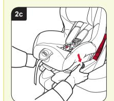
Press the safety buttons on the left and right side of the seat base together (dia 2c). TIP - This ensures that both hooks on the locking arms are open and ready to use.
