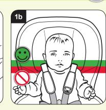
Your child's head MUST be centralised within the headrest (dia 1b). The shoulder strap slots in the cover and shell MUST be level with the top of your child's shoulders. If in any doubt always position the slots slightly above the shoulder rather than below it (dia 1b). However, once you reach the top position your child may continue to use the seat until their eye line is above the top of the seat shell or their weight exceeds 18kg.
