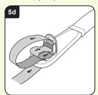
Remove the chest pad strap from the chest Feed the harness strap all the way out of pad attachment arm. Pull the chest pad the **SAFESTRAP™** mechanism until it is strap through the shoulder strap slots to the released (dia 5d).
