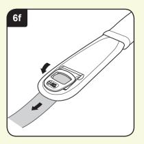
Pull through all the excess slack to close the indicator (dia 6f).
