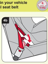
Engage the buckle tongue in the vehicle seat buckle. CLICK! Place the lap belt section in the lap belt routing guides on both sides of the seat
