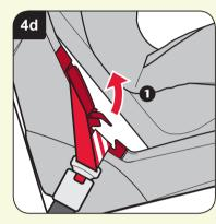
Whilst holding the diagonal belt tight pull up on the clamp lever **1** until it engages (dia 4d).
