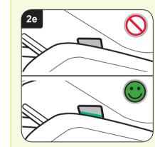
IMPORTANT – The green markings on the safety buttons must now be visible on both sides (dia 2e).
