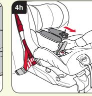
The child seat should now be secure. To check pull forward firmly on the harness. There should be little or no movement (dia 4h).
