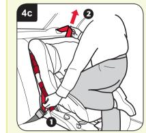
**IMPORTANT** – Do not twist the belt Firmly push the child seat into your vehicle seat using your body weight. Pull and hold the diagonal belt **1**. Pull at **2** to remove all **IMPORTANT** – Do not twist the belt.
