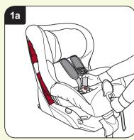
Harness adjustment With one hand press the adjuster button and with your other hand **BELOW** the chest pads, pull both shoulder straps forward as far as possible to loosen the harness (dia 1a).
