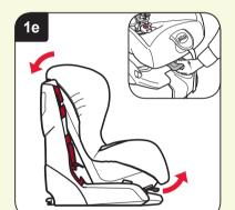
Reclining the child seat The child seat can be used in either an upright, or reclined po Squeeze the recline handle (dia 1e inset), underneath the front of the child seat, and slide the child seat shell into the desired position.
