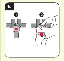
Unfasten the buckle by pressing the red harness buckle button **(dia 1c)**. To fasten the buckle; first fit the two upper sections together, then push them firmly into the lower section until you hear a positive "CLICK" **2**.
