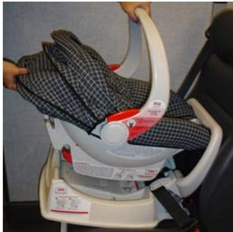
Remove infant carrier from base. The base can remain in the vehicle during visual inspection of carrier.
