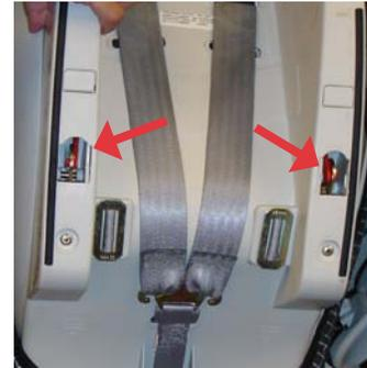
On bottom of carrier where rubber strips run along edges of support rails, there is an exposed opening with attachment hooks.
