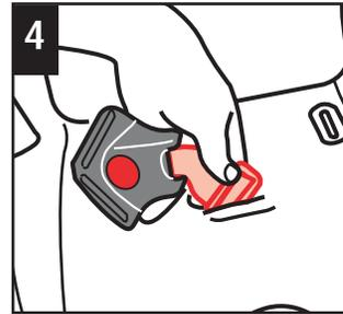
4 Rotate metal clip, then insert up through the shell and pad. From the front, pull buckle free from shell and pad. Lock buckle plates into buckle for future use.
