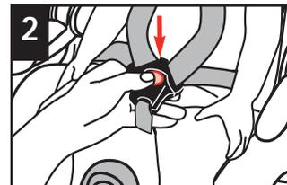
2 Press red button on buckle to release the buckle plates.
