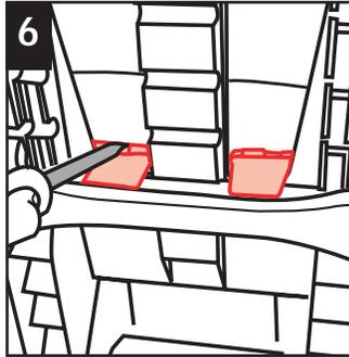
From the back, use a screwdriver to press in on lip of upper harness guides and pop guides through the front. Pull cover off headrest.
