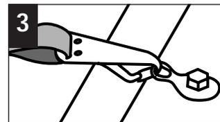
3 With knee still in child restraint, attach hook to anchor in vehicle. Push down firmly and tighten top anchorage strap.
