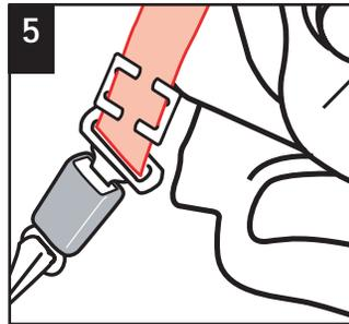
5 Rebuckle belt. Lap belt portion should now be tight. If not, remove locking clip and repeat all steps.
