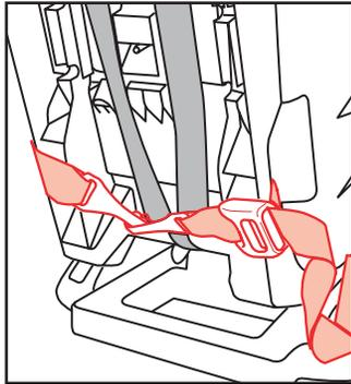
When LATCH is not being used, fasten belt hooks together behind the child restraint as shown.
