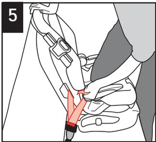
**5** Place one knee in the child restraint and push down firmly while pulling up on the loop to tighten belt.
