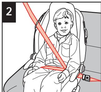
**2** Place BOTH shoulder and lap belt across child's thighs. Lock buckle. **NOTE:** Make sure the lap and shoulder belt are placed under armrest as shown.
