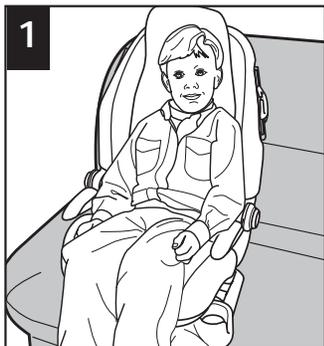
**1** Child restraint must be in the full upright position. Pull out on recline handle and pull child restraint all the way up. Place booster seat against the back of the vehicle seat. Tuck the top anchorage hook and splitter plate under the base. Have child sit in seat with his back and bottom fully in the seat.
