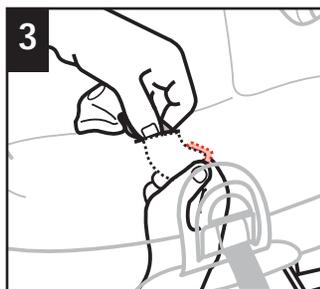
3 With seat reclined all the way back, reach under seat between base and shell and locate buckle's metal clip. It will be flush against the shell.
