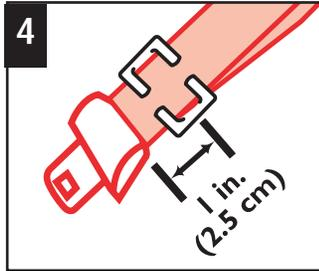
4 Position locking clip about 1 in. (2.5 cm) from vehicle belt's buckle plate.
