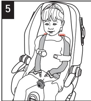
5 Place the child's bottom and back flat against the child restraint. This will increase comfort and allow the harness to properly tighten.
