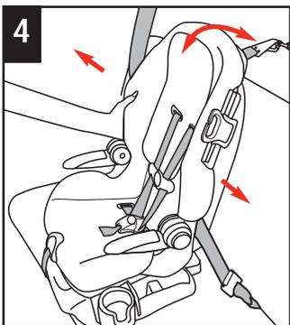
With weakest hand at belt path, tilt and push the child restraint forward and back, and from side to side. If the seat belts do not loosen, your child restraint should be secure.
