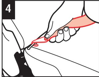
**4** Fasten one LATCH belt hook to the anchor in the vehicle seat located in the vehicle seat bight. Repeat for other side of child restraint. See your vehicle owner's manual for locations and more information.
