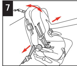
**7** With weakest hand at belt path, tilt and push the child restraint forward and back, and from side to side. If the LATCH belts do not loosen, your child restraint should be secure.
