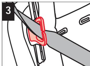
**3** Secure the vehicle shoulder belt through the notch in the shoulder belt guide. The belt should cross the base of the child's neck and across the chest (not the face or neck). Pull up on the vehicle shoulder belt to tighten.
