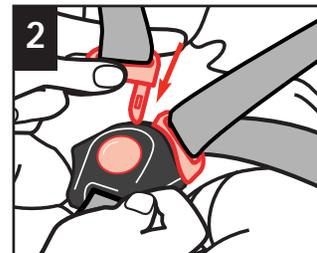
Push each buckle plate into buckle until you hear a "click". Remember to always pull up on harness straps to make sure buckle is locked tightly.
