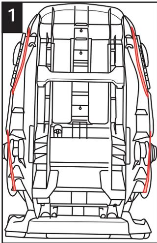
1 From back of shell, release the elastic straps shown in red.
