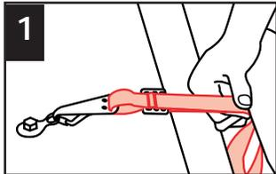
**Style 1 - To Attach Top Anchorage Strap:** Put knee in child restraint and push down; attach hook to anchor in vehicle to estimate how much adjustment you need, then unhook.
