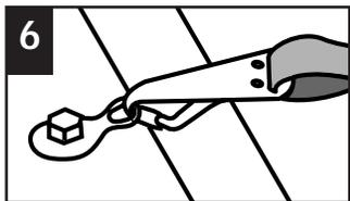
**6** With knee still in child restraint, attach hook to anchor in vehicle. Push down firmly and tighten top anchorage strap.
