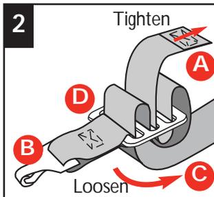
**To Adjust Top Anchorage Strap:** Loosen top anchorage strap into "loops" at adjuster slide as shown above.
