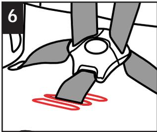
6 **Adjust Buckle:** Determine which of the three available buckle slots is both comfortable and snug. Refer to "Removal of Harness" to adjust buckle.
