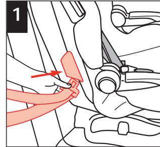
1 Connect and tighten harness straps prior to installing in vehicle.
