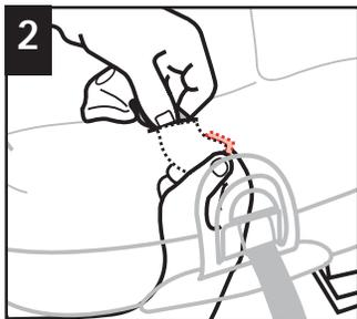
**2** With seat reclined all the way back, reach under seat between base and shell and pull buckle clip through pad and shell. Make sure buckle clip is flush against bottom of shell.
