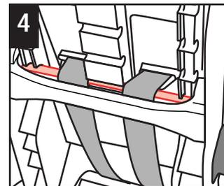
**4** Pull harness through the back. Make sure the harness goes OVER the metal bar, BETWEEN metal bar and plastic handle of the harness/headrest adjuster.
