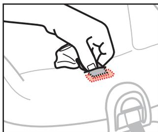
Failure to place buckle's metal plate completely through pad and shell can result in serious injury or death to the child.
