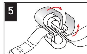
**Style 2 - To Attach Top Anchorage Strap:** At the adjuster, unlace free end of strap from right side of adjuster slide and loosen into "loops" (1). Put knee in child restraint and push down; attach hook to anchor to estimate how much you need, then unhook (2).
