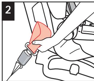
Grasp both vehicle belts together just behind the buckle plate and unbuckle. **NOTE:** If the buckle plate ends up behind the child restraint, grasp the belts to the outside of the child restraint, as close to the buckle plate as possible.
