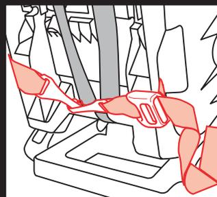
Do not use LATCH when using the Belt-Positioning Booster.
