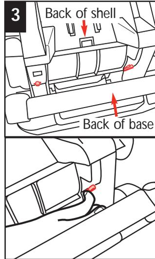
3 Remove both lower harness guides in bottom of seat by reaching between the base and shell from the back.
