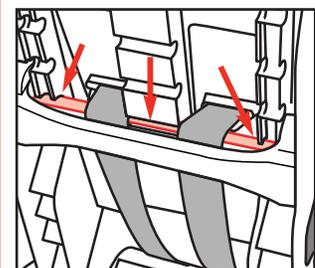
**Make sure metal bar is locked into position. Failure to do this can result in serious injury or death.**
