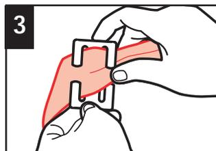
Thread both portions of the vehicle belt onto the locking clip.
