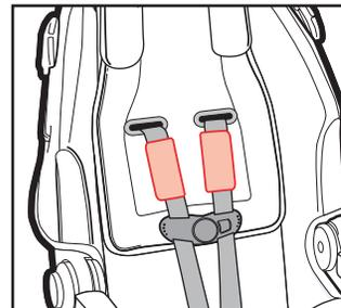
**Harness Covers (on select models):** Harness covers help provide comfort to the neck. For Harness Covers to fit correctly, you may have to fit the upper ends of the covers through the harness slots. To remove the covers, unthread the harness from harness bracket (see belt-positioning booster section), remove covers, and rethread harness. Reverse to replace insert.
