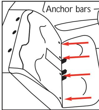
LATCH means **L**ower **A**nchors and **T**ethers for **C**hildren. Not all vehicles manufactured before September 2002 were equipped with LATCH.
