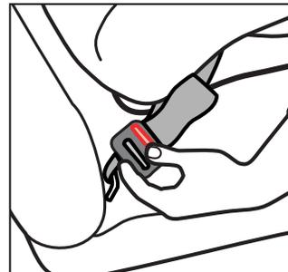
**To release LATCH:** Remove child from child restraint. Press down firmly on adjuster side of child restraint and press release button to release tension. Unhook LATCH from bar by squeezing spring lever and twist hook off bar.
