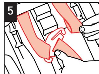
**5** Fit loops on harness ends onto the splitter plate.
