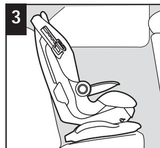
Connect and tighten harness straps prior to installing in vehicle. Place child restraint **flush** against the back of the vehicle seat **forward-facing** in the back seat.
