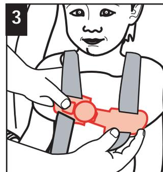
3 Press on release button and pull apart. Place harness over sides of child restraint. Remove child.
