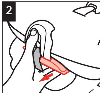
To fully recline, pull out on handle and push top of child restraint back.
