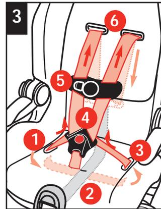
**3** Thread one end of harness down through slot on left side of shell (1), across bottom of seat (2) and up through slot on right side (3).
