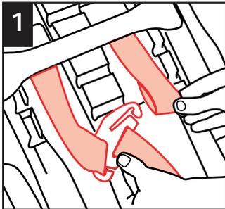
1 From the back of the seat, unfasten harness from splitter plate.
