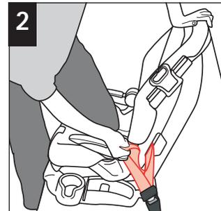
2 Place one knee in the child restraint and push down firmly while pulling up on belt to tighten. For a manual belt, refer to "Knowing your Vehicle Belt" section.
