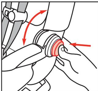
Depending on your model, your child restraint may have a red button which will lock the armrest in either the upright or down position. To rotate locking armrests, push in on red button and rotate. Make sure armrests lock into place.
