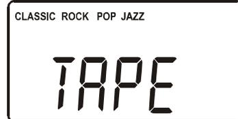
To change the EQ setting press the **EQ** button on the top panel until the desired setting appears in the display.
