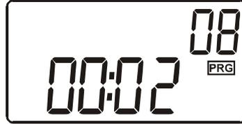
After the last programmed track has played the player stops but the programmed tracks remain in the memory. To play the programmed tracks again, press the **PROG. ↻** button and then the **PLAY/PAUSE ►||** button.
