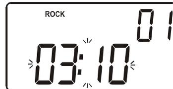
Press the **PLAY/PAUSE** ►|| button once more to cancel Pause mode and resume playback. The elapsed time display stops flashing.
