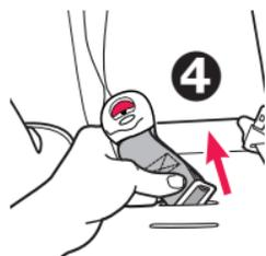
5. Pull on the adjustment strap ⑤ on the front of the seat to lock the metal junction plate into place.
