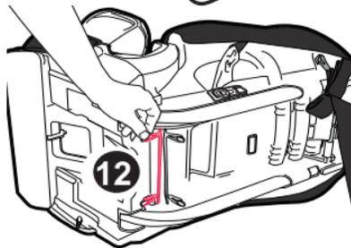
14. Pull elastic strap on the seat pad through the vehicle belt guide on side of seat and attach to hook as shown. Repeat on other side **13**.
