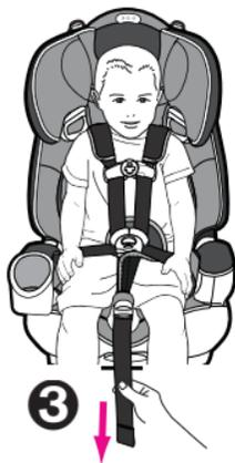
5. Make sure straps are flat and snug against child's shoulders and thighs. You should not be able to pinch **4** the harness straps. A snug strap should not allow any slack. It lies in a relatively straight line without sagging. It does not press on the child's flesh or push the child's body into an unnatural position.
