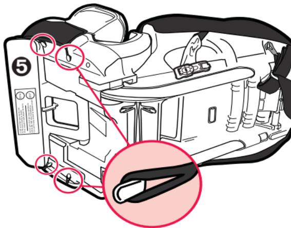
5. Pull elastic loop on the seat pad through the vehicle belt guide on side of seat and attach to hook as shown ⑥ . Repeat on other side.
