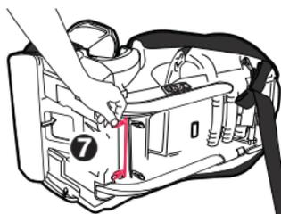
8. Also detach the elastic straps that are threaded through the vehicle belt guides on the sides of the seat as shown in ⑧. Repeat on other side.
