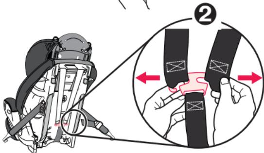
3. Remove crotch strap by pushing the strap retainer ❸ on bottom of seat, up through slot.
