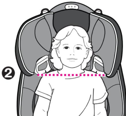
To adjust head support side wings, push buttons on top of seat down and rotate wings to desired position.
