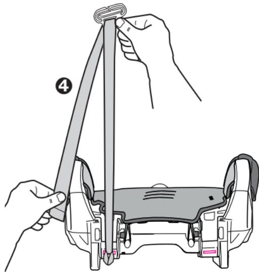
4. Slide the vehicle shoulder belt onto the clip as shown ⑤ and pull free end of strap down ⑥ to tighten clip against the child's shoulder.
