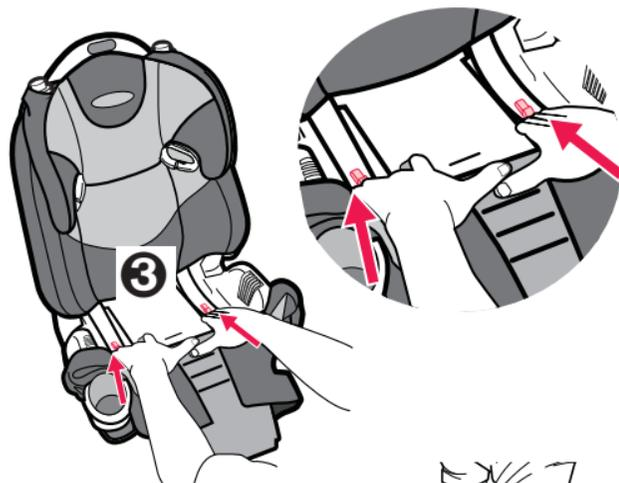
4. Move seat pad fabric out of the way and squeeze red buttons together to release back support from seat. Pull seat and back support apart ④.
