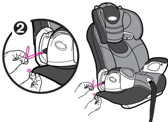
3. Pull the seat pad out of the way to reveal red buttons as shown in ③. Slide the buttons to release the back support from the base and lower it into a flat position.
