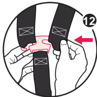
10. Reassemble straps onto metal junction plate exactly as shown **12**.
