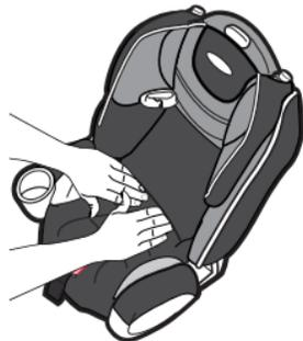
13. Attach 2 seat pad elastic straps onto the hooks on the rear of the child restraint as shown in **12**.
