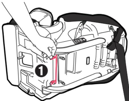
2. Detach elastic strap from the hooks on the seat pad as shown. Repeat on other side **2**.
