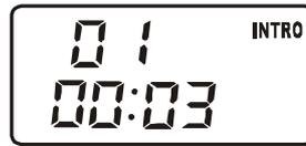
To cancel Intro Scan press the Stop ■ button or press the MODE button until none of the special playback mode indicators appear in the display.
