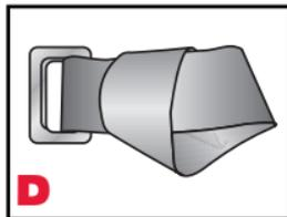
Because every vehicle model is different, sometimes you cannot find a location to properly anchor the tether, or the structural part of seat is too large for the hook. Use rear-facing tether connector strap (fig. D) to assist in creating an anchor point.
