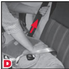
8 Verify all connections are secure and that restraint is stable. The restraint is secure when it cannot be moved front-to-back or side-to-side more than 1" (2.5 cm.) at belt path. If the restraint is not secure, repeat procedure or use an alternate seating location.
