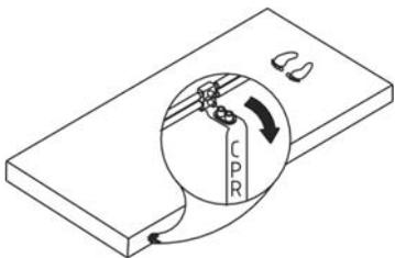
When there is an emergency to perform CPR on the patient, quickly pull the CPR valves to release air from mattress. The CPR valves are located at the head-end, right-hand-side of the mattress. The quick connector found from the pump unit can be disconnected for even faster deflation.
