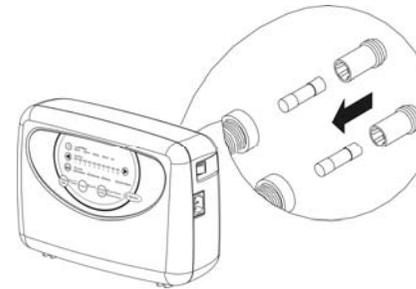
1. Disconnect the plug form mains power when a blown fuse is suspected.
