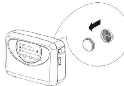
1. Loosen the screws from the air filter plate located at the back of pump.
