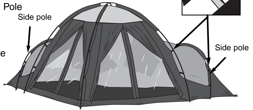
illus. 6 Assembled tent without Rainfly. Note the Frame Clips located on tent.
