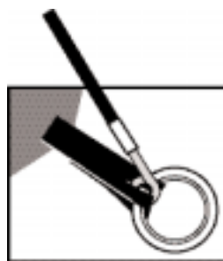
illus. 3 Insert pole end onto pin & ring
