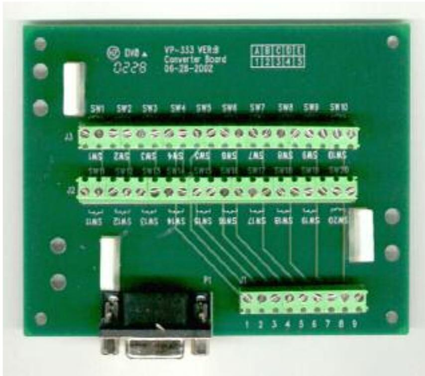
The beauty of the card is that it makes the switch wiring simple if you are building a push button controlled, multi track video kiosk or display.
