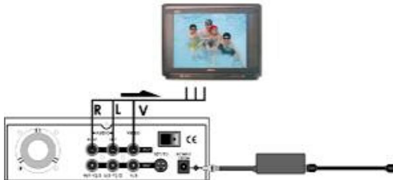
To connect to a SCART input, a three phono (RCA) plug (Left and Right Audio plus Composite Video) to SCART Plug cable will be required.
