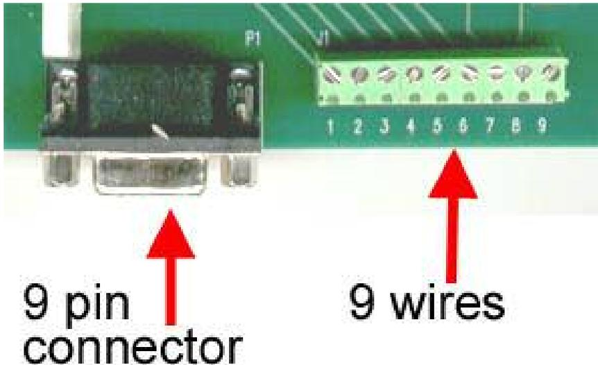
You may connect either a 9-pin connector or nine wires.
