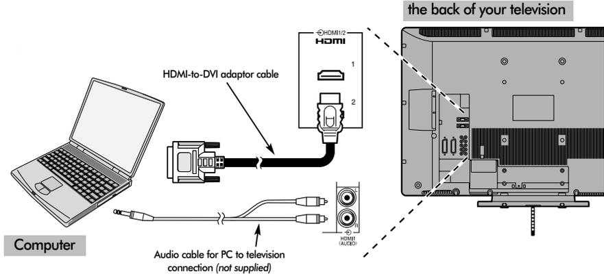
When connecting a PC to the HDMI terminal on the television, use an HDMI to DVI adaptor cable and an analogue audio cable.
