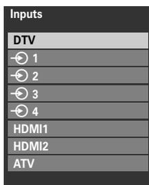
HDMI displays equipment connected to *Input HDMI* on the back of the television.
