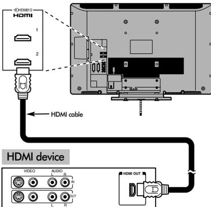
To view the HDMI device video, press the
