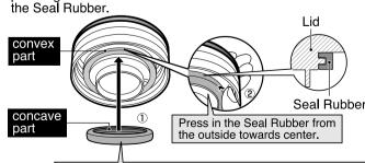
As there is no difference on the surface of the Seal Rubber it can be attached whichever side facing up
