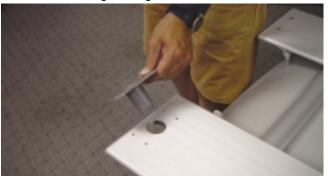
Use four 3/4" screws to attach each flush mount adapter to the aluminum slat with a phillips head screw driver. Please note, the adapters can stay attached to the slats and never need to be disassembled.
