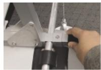
(3) Push the snaplock bracket so that the pin is snapped in position.
