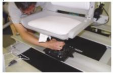
Please note, for disassembly it is very easy to detach the swivel seat or the pedestal from the quick release seatmount by sliding them out while lifting up the spring loaded quick release lever mechanism on the swivel seat mount with your finger as shown below.
