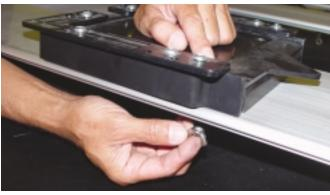
Now slide the swivel seat(s) into the quick release swivel seat mounts and <u>make sure that the spring loaded lever</u> <u>mechanisms locks in place</u>.
