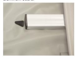
Similarly, slide the long stabilizer underbars from the stern of the FoldCat under the rearmost, 2nd rearmost and the 3rd rearmost aluminum slats.
