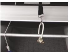
The center black strap on the canopy should be attached to the sea tie on the aluminum step rod in the bow.
