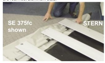
Align the stern ends of these underbars against the triangular markings on each pontoon in the stern.
