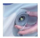
Put the new outer valve in place and tighten by hand until secure. Use the black Halkey-Roberts valve replacement tool to tighten completely.
