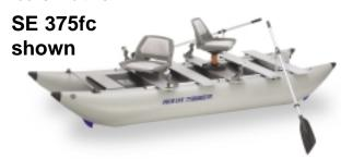
Please note, after first time assembly of the FoldCat 325fc or 375fc, for disassembly all you have to do is deflate the air chambers, remove the underbars, swivel seats, rodholders, oars and unscrew the oarlocks. For transportation, simply roll-up the hull along with the aluminum slats & motormount and place it in the FoldCat carry bag.
