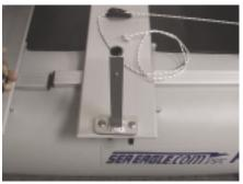
Install the two raised oarlock bases on the sides of the second wide aluminum slat from the bow as shown.
