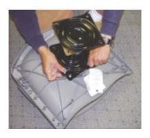
Bolt the upper end of the pedestal to the swivel seat as shown above. And then slide the other end of the pedestal into the quick release swivel seat mounts and <u>make sure</u> that the spring loaded lever mechanisms locks in place.
