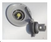
The valve cap unscrews to reveal the yellow valve stem. When this stem is in the up position as shown the valve retains air. The valve should be in this position to inflate the boat.
