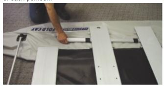
Align the bow end of the stabilizer underbar against the triangular marking on the bow of each pontoon as shown below Please note, on the SE 325fc, the 2 short stabilizer bars actually are closer to the aluminum board than shown above and they should meet together under the center aluminum board.
