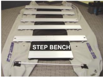
Feed the 2 fabric beads in the bow of the 375fc FoldCat hull through the 2 nylon slotted fittings under the aluminum step bench as shown.
