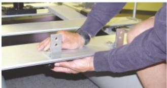
Secure the wooden motormount plate to the L-brackets by running the other 2 bolts through the top holes in the L-brackets and the 2 holes in the motormount plate itself. Tighten all knurled nuts and bolts.
