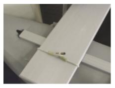
Then install the other 2 Sea Ties to the last slat in the stern of the FolCat as shown.
