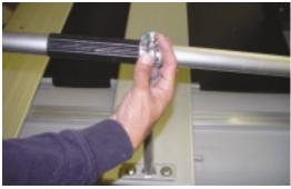
On the 325fc, the raised oarlock bases are installed on the first aluminum slat in the bow. And then attach the oarlock pins and oars as explained above for 375fc.
