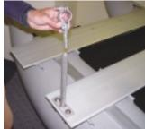
Now snap the two 8' sectional oars together and inset each oar into the oarlock pins and tighten the wingnuts to secure the oars as shown below.
