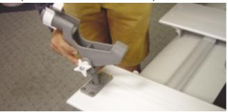
For disassembly, you only need to detach the rod holders from the flush mount adapters.
